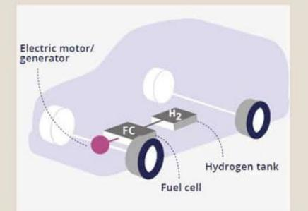
Fuel cell electric vehicles use a fuel cell to create on-board electricity, generally using compressed hydrogen and oxygen from the air.
